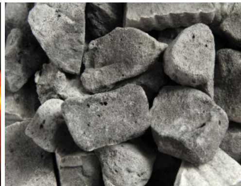
Upon cooling, the foam glass cake breaks through tension cracks into foam glass gravel.
